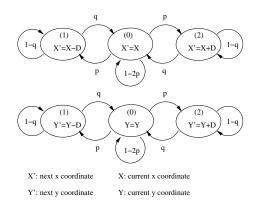
Fig. 3. State transition diagram for the SIMM model
